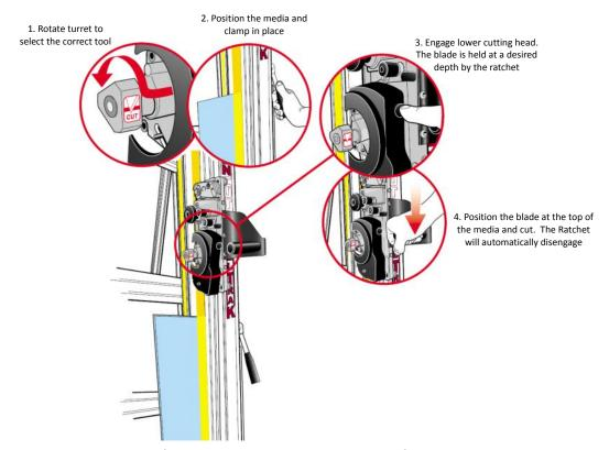
\*Note - Do not cut PVC Foamboard too fast. At the correct speed a smooth 90° finish will be achieved; cutting too fast will result in a rough and unacceptable edge.
